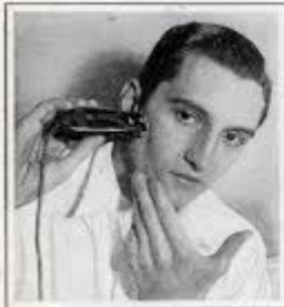
Operating on the principle of a barber's clippers, this electric razor gives a clean shave without use of lather.
